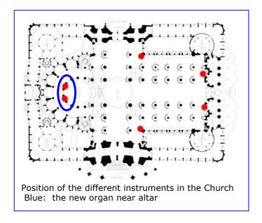
This solution achieved an unusual stereo effect sound, instead of the usual organ sound coming from a single focal point. Sound originating from different points causes a surround-sound, stereophonic or 3D effect for the listener which strengthens the architectural space and omnipresence of the divine message.
